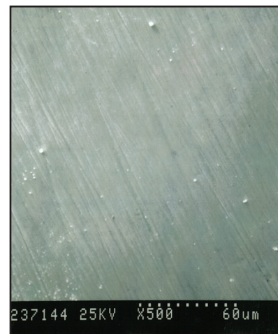
Figure 5 - Scratches Produced By 400 Grit StaiNo ® Tooth Stain Eraser SEM Magnification 500X
